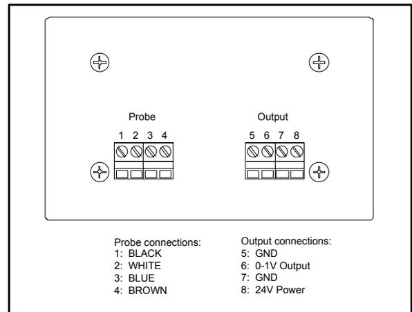
**Figure 3. Display unit connections**
