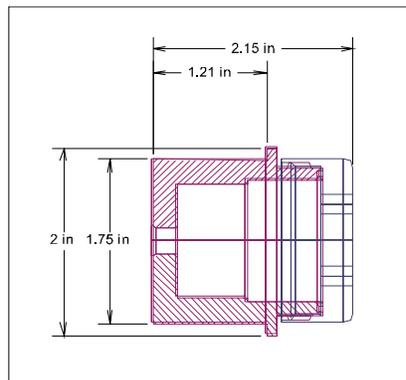
*Figure 1. Probe dimensions*
