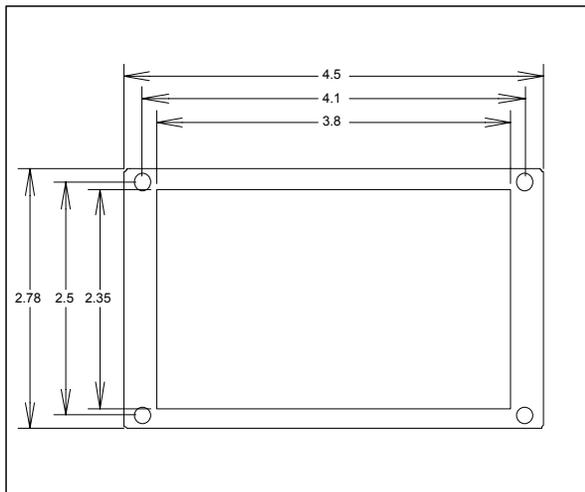
**Figure 4. Display unit panel cut out**
