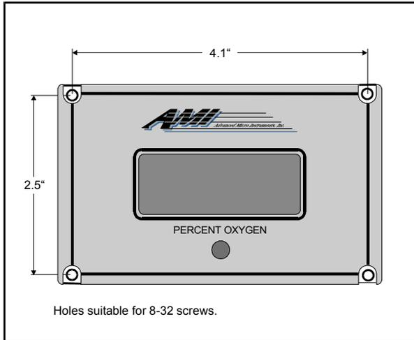
**Figure 2. Display unit showing mounting hole dimensions**
