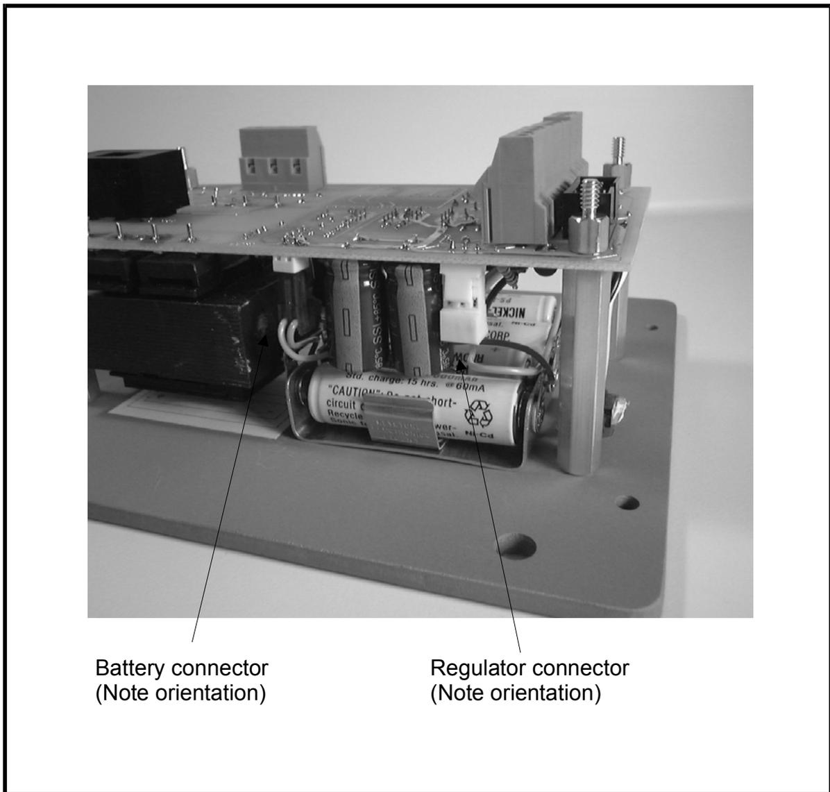
*Figure 3. Location of battery connections*
