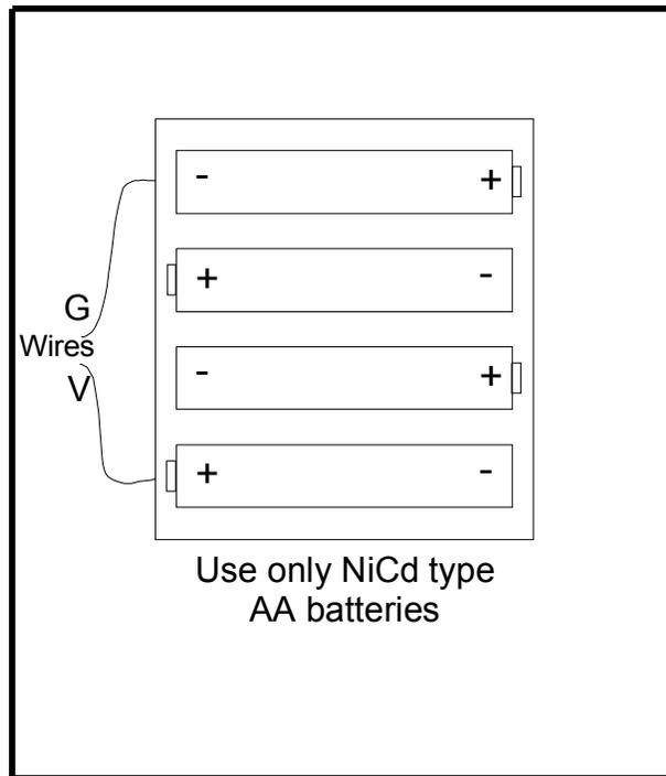
*Figure 4. Battery orientation*
