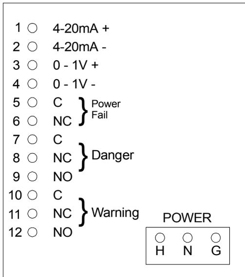
*Figure 2. External connections.*
